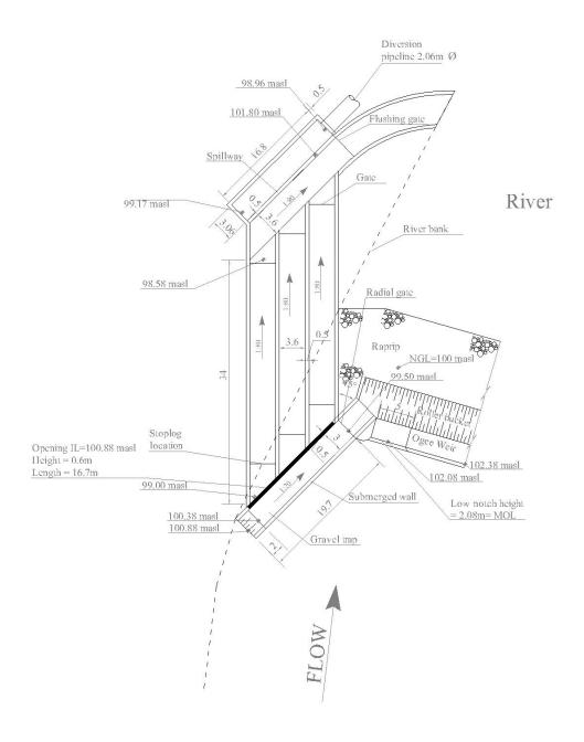
Figure 2 Mitchells Pass Diversion at 5m<sup>3</sup>
