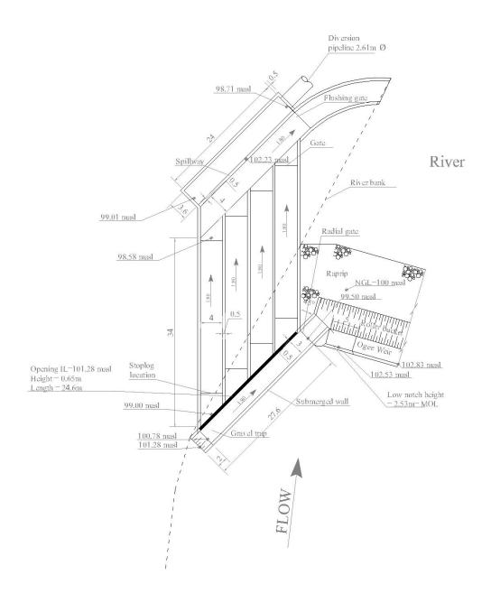
Figure 3 Mitchells Pass Diversion at 8m<sup>3</sup>
