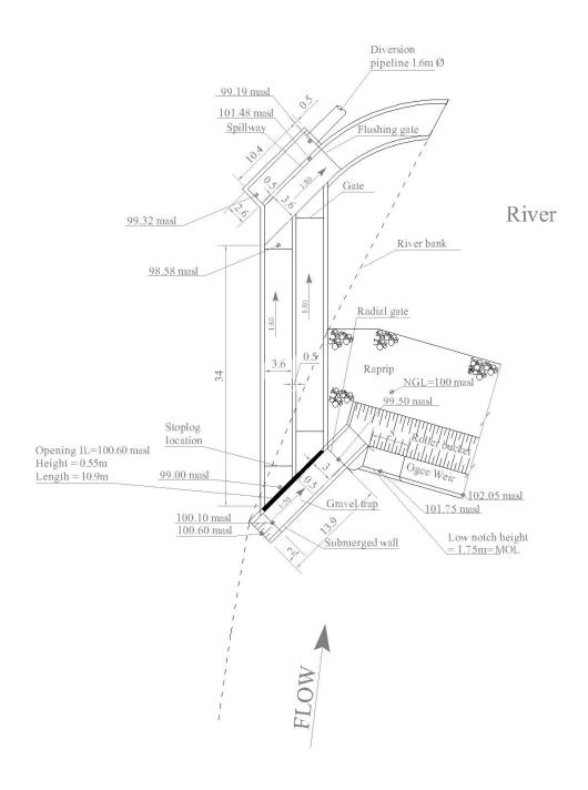
Figure 1 Mitchells Pass Diversion at 3m<sup>3</sup>
